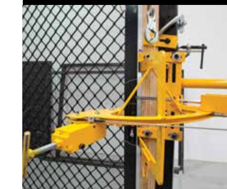
This internal test simulates an attack with a screwdriver.
